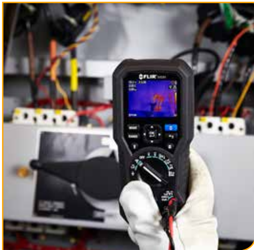
电气面板的热扫描
